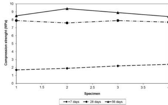
**Figure 3.** Compressive strength for different curing times using cement dosage of 600 kg m<sup>-3</sup>.
