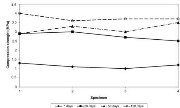
**Figure 1.** Compressive strength for different curing times using cement dosage of 200 kg m<sup>-3</sup>.
