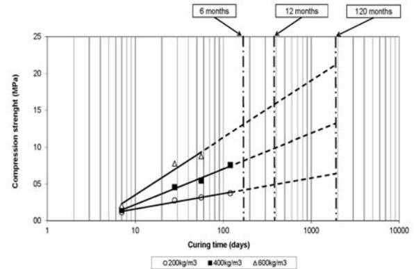
**Figure 7.** Compressive strength versus curing time.
