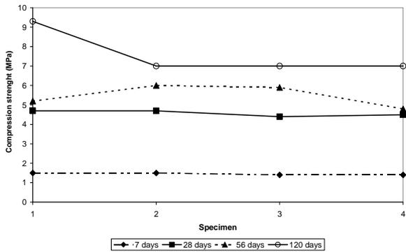
**Figure 2.** Compressive strength for different curing times using cement dosage of 400 kg m<sup>-3</sup>.
