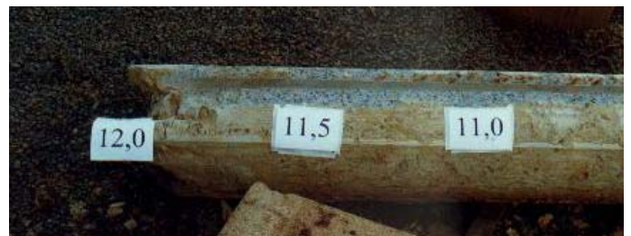
Figure 7. Detail of the CFA pile tip.
