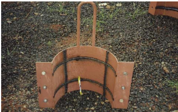
Figure 4. Arrangement to fix the pile.
